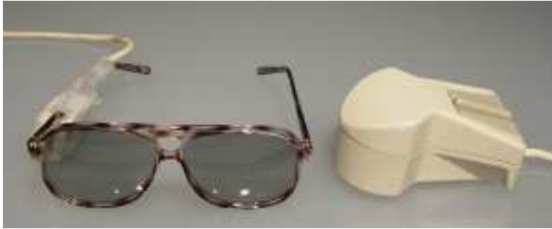
Figure 5.2: Circularly polarized lenses with a tracker on the side as well as a 6DOF mouse with three input buttons
